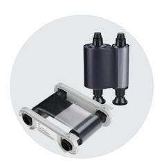
The Evolis High Trust<sup>®</sup> KO ribbon has been specifically engineered to bring durability to monochrome personalization. The KO ribbon has 2 panels; a black panel (K) to print black text or barcode, and a clear overlay panel (O) to apply a thin protective film.
